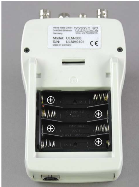
Fig. 2 Polarity of the batteries
