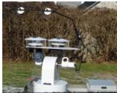
SMT in typical BSRN mode with SDK, PIR, SPP and sNIP
