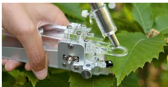
Leaf Clip with Laterally Mounted Coaxial SMA Socket for Additional Light Sensor
